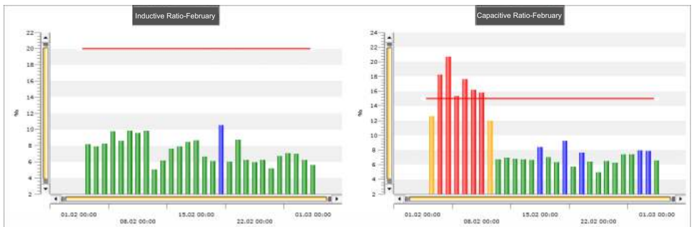
Monthly graph of inductive and capacitive rates of a power factor correction panel
